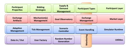
**Fig. 1.** Conceptual Framework of a Simulation Environment for Autonomic Markets a testing environment for the future studies. Fig. 1 illustrates the layers and components of our proposed simulation architecture, which are as follows:
